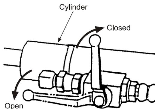
CAUTION: close the stop valve, and be sure stop the engine to prevent danger during inspection.
