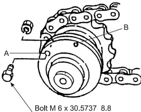
When the shear bolt is served stop the engine and remove the causes and replace the bolt.
