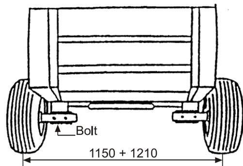
Wheel tread is adjustable with bolts and nut indicated.
