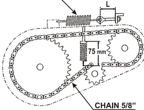
ADJUSTMENT OF ROLLER CHAIN TENSION
