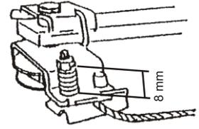
ADJUSTMENT OF PICK-UP CHAIN AND SUSPENSION
